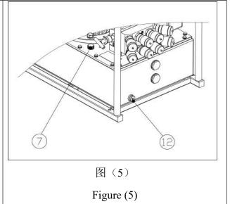
Detailed operations: Open the oil filler and ventilator plug (7) on the hydraulic pump, unscrew the drainage plug (12) from the side drainage port of oil tank to fully drain the hydraulic oil into an appropriate container, and then clean and reinstall the drainage plug (Figure 5).
