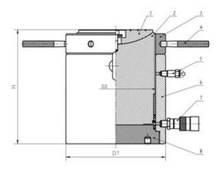
1 - <u>Saddle</u> 2 - Piston rod 3 - Lock nut 5 - Handle 5 - <u>Safety</u> valve 6 - Cylinder 7 - Quick coupling 8 - Bottom cover
